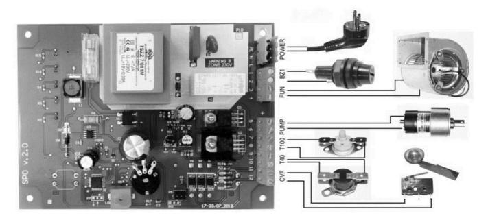
Fig. 1. The connection of the universal oil heater type MTM15-35GT.
