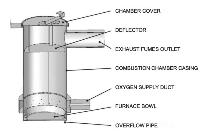
Fig. 6. Combustion chamber
