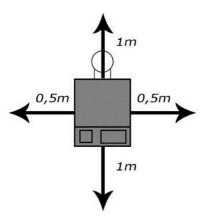
Fig. 2. Minimal safety space around the device.
