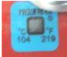
Figure 5.19. View of the irreversible thermosticker, used to mark an alarm overheating of the pellet's delivery pipe – activated condition, the active segment is dark, the temperature has exceeded activation level of 104°C;
