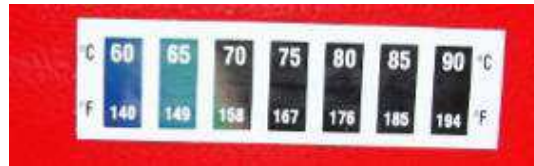
Figure 5.15. View of the reversible thermosticker, used to measure the spot temperature – condition at increased burner's body temperature – in the range of 60 – 65°C;
