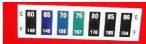
Figure 5.16. View of the reversible thermosticker, used to measure the spot temperature – condition at increased burner's body temperature – in the range of 70 – 75°C.
