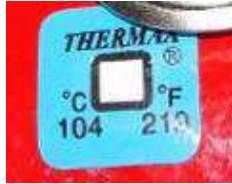
Figure 5.18. View of the irreversible thermosticker, used to mark an alarm overheating of the pellet's delivery pipe – initial condition, the active segment is white, the temperature has not reached activation level of 104°C;
