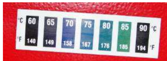
Figure 5.17. View of the reversible thermosticker, used to measure the spot temperature – condition at increased burner's body temperature – in the range of 80 – 85°C.
