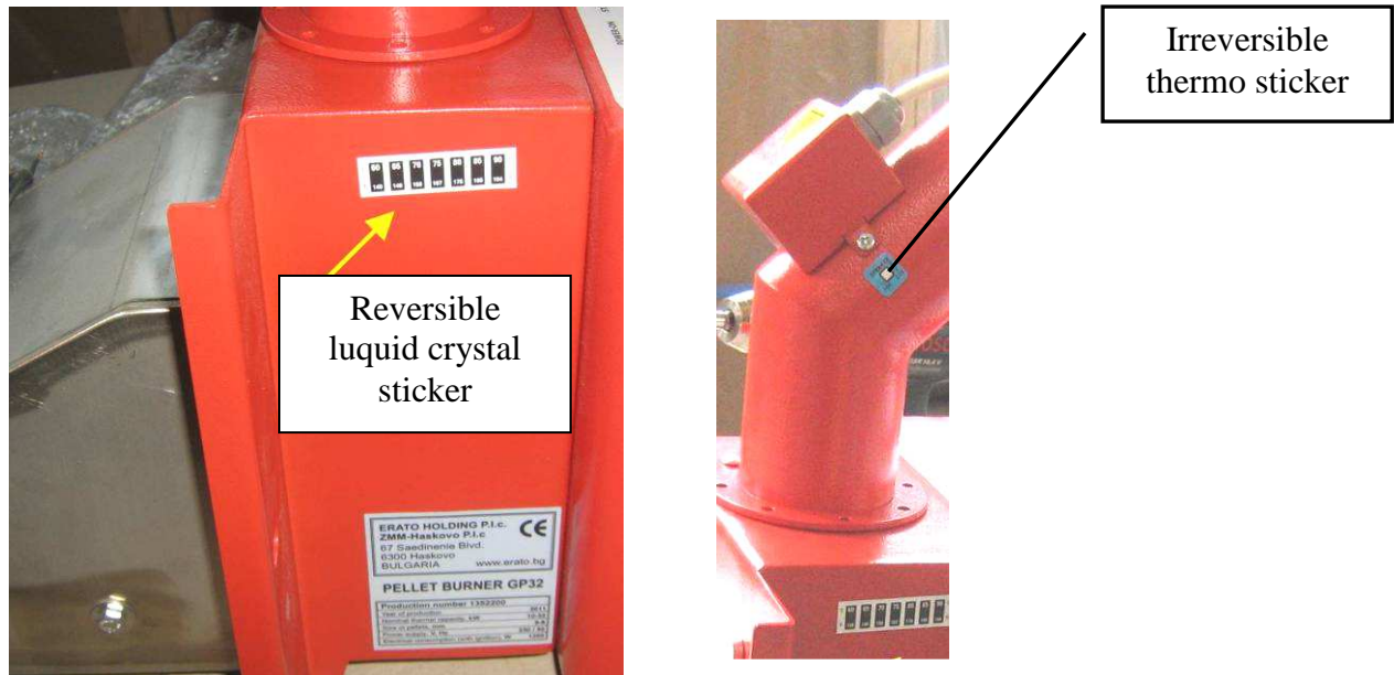
Figure 3.4. View of the side of the burner with attached liquid crystal thermo sticker;
