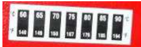
Figure 5.14. View of the reversible thermosticker, used to measure the spot temperature – initial condition, at normal room temperature;
