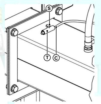
Fig.22. Feeder temperature sensor installation.
