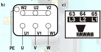
Fig. 11. a) gear-motor, b) motor connection terminals with cover removed, c) controller terminals used for connecting the gearmotor.
