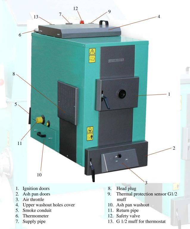
Fig. 1. Moderator-type boiler (version designed for use in ABB set) – main parts.
