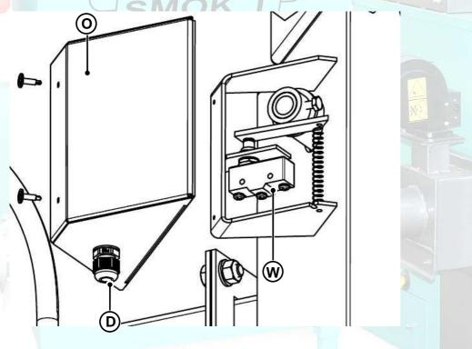
Fig.27. Location of the limit switch
