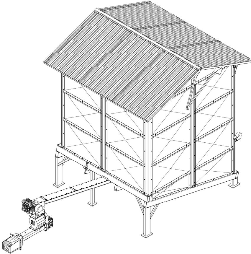
*Fig. 1.6. APSB set with a 27 m<sup>3</sup> container and a 40 kW cast iron head.*
