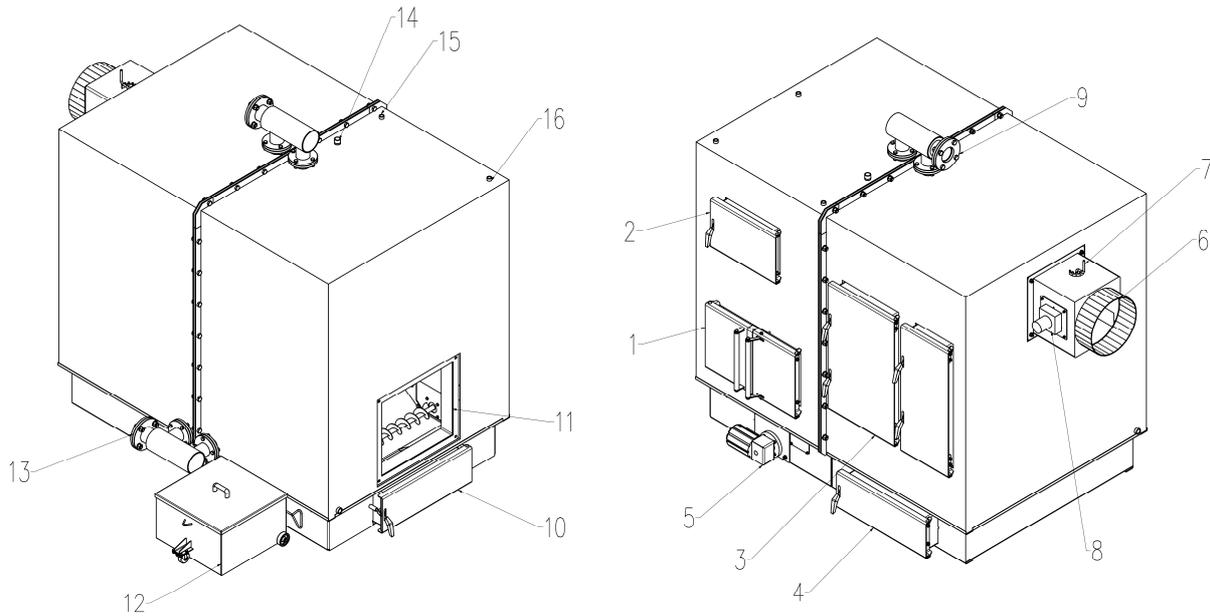
*Fig. 1.3. 180, 240 kW Moderator exchanger - main elements.*
