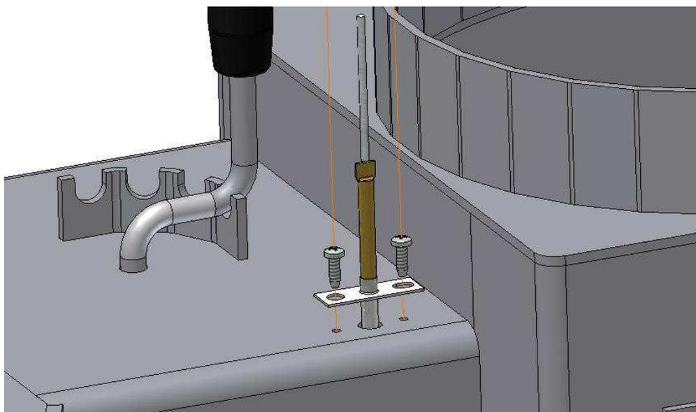
*Fig.2.9. Exhaust gas temperature sensor installation.*
