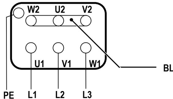
*Fig.2.4. Connection terminals inside the feeder motor junction box.*
