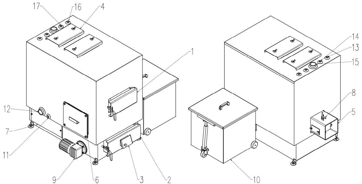
*Fig. 1.1. 60 kW Moderator exchanger - main elements.*
