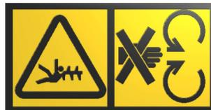
The transport worm may start operating without warning. Switch off power supply before lifting the cover.
