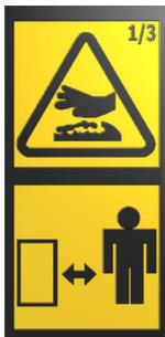
Pay special attention in the boiler room keeping in mind that various parts of the boiler and systems may be hot. Keep a safe distance.
