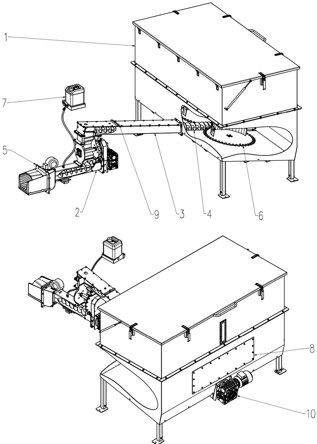
*Fig. 1.4. APSB set with a 4 m<sup>3</sup> container and a 40 kW cast iron head*
