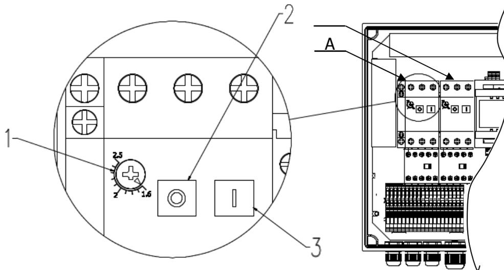
*Fig.2.5. FEEDER MOTORS PROTECTIVE SWITCHES*
