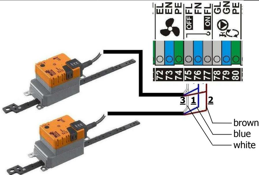
Fig.2.6. 180 and 240 kW - Belimo actuator connection diagram
