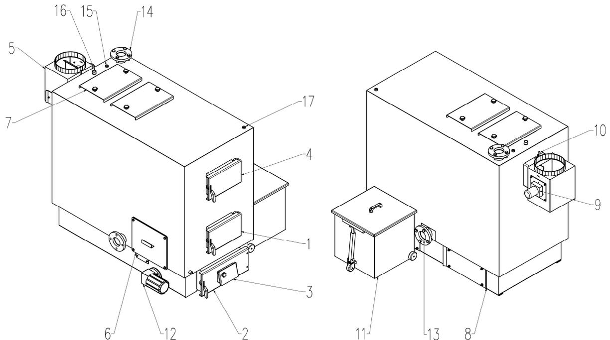
*Fig. 1.2. 120 kW Moderator exchanger - main elements.*
