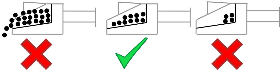
Fig.3.1. Proper level of fuel
