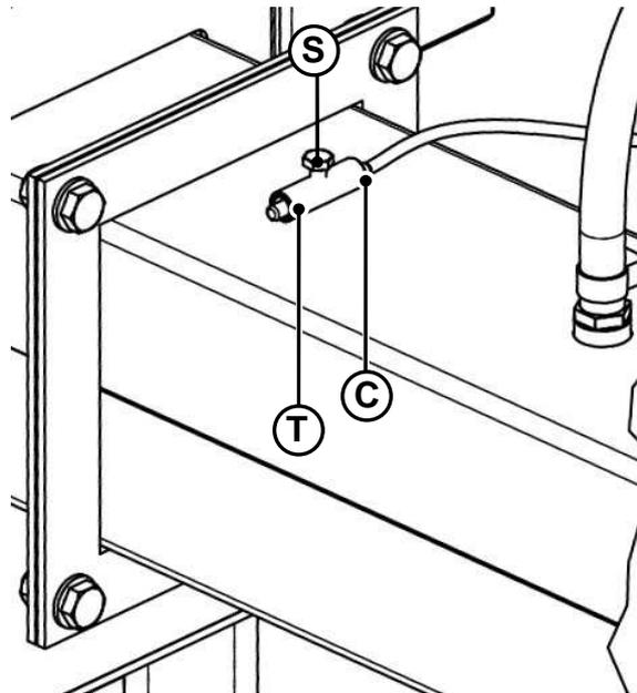
*Fig.2.8. Fuel feeder temperature sensor installation*
